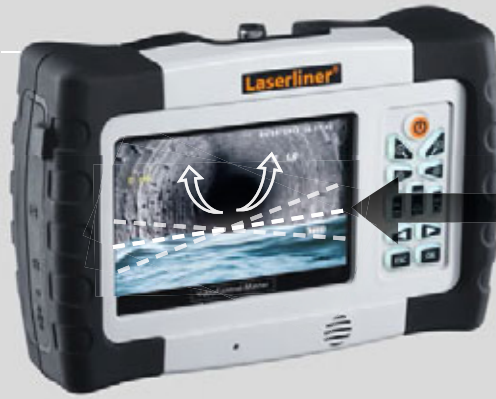
LevelFlex: Horizontal self-alignment for optimum image playback
